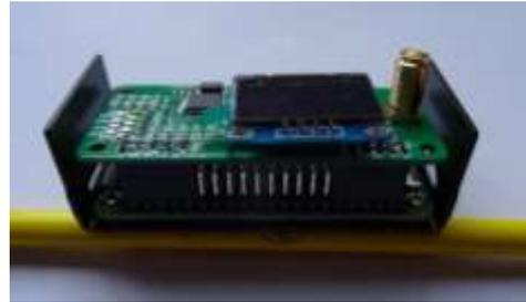
Then, using the two spacers and the two longer screws, bolt through both boards into the base. Once all four screws are located, they can be tightened properly.
