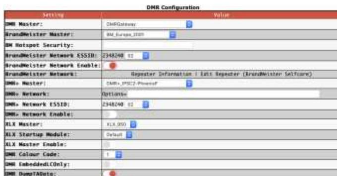
If you use the dashboard to turn on a specific Network, by turning off the ones you don't want, you can listen to one Network at a time. In Brandmeister mode you can connect, say, to TG 3211 and it will work. Alternatively, in Phoenix mode you can use TG 235. However, if the radio Network selection is out of step with the Hotspot, then it might not!
